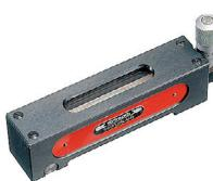
For measuring irregularities of plane surfaces, measuring range  $\pm 5$  mm, with wooden box.
