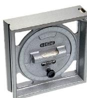
With fine setting device, two flat bases and two prismatic bases, with circular scale, division of 2 x 180 deg., vernier for reading at 3 arcmin, with wooden box.
