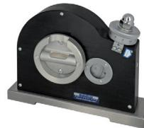
Instrument for measuring angular deviation accurately, with circular scale 2 x 180 deg., with finely ground prismatic base of hardened steel for measuring on shafts and flat surfaces, with micrometer graduated 1 Div. = 1 arcmin, with wooden box.
