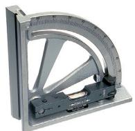
With fine setting device, with 2 prismatic bases, allows easy checking of angles up to 90 deg. in degrees and minutes, vernier for reading at 10 arcmin, with wooden box.
