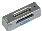
Horizontal spirit level with slot windows which enable the view on the vial from the side. Standard version with prismatic measuring base, not recessed in the middle part, with wooden case.
