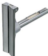
With removable tubular level, prismatic measuring base 150 x 40 mm for vertical measurements, flat face of the tubular level 150 x 10 mm for horizontal measurements, with wooden box.
