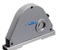
The CLINORAPID 45 is suitable for measuring any inclination in degrees and minutes, on flat surfaces and shafts. Measuring range ±180 degrees. As this instrument does not measure using a glass vial, it is nearly independent from the environmental temperature and can therefore very well be used for outdoor measurements.
